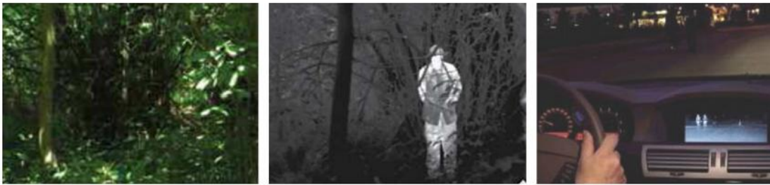
Fig. 2. Visible image (left), same image in the infrared (center), night driving assistance (right).
